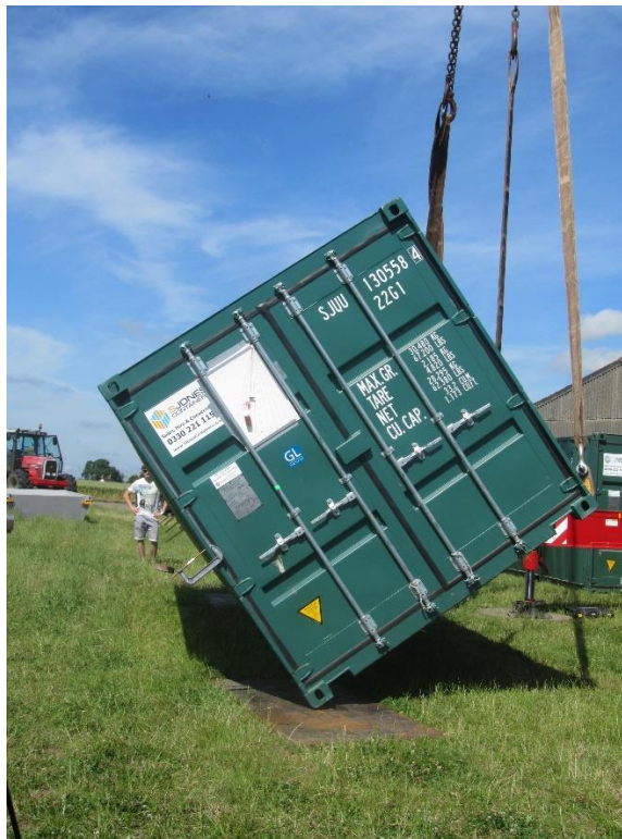
Figure 4. Rotating the container. Protractor and plumb bob on LH door
